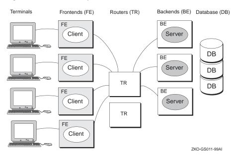
Figure 2–1 The Three Layer Model
